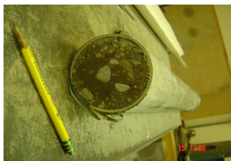
Extrude sample from tube
