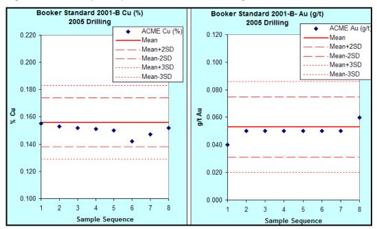
Figure 13.3 Sample Sequence Charts – 2005 Drilling Standard 2001-B
