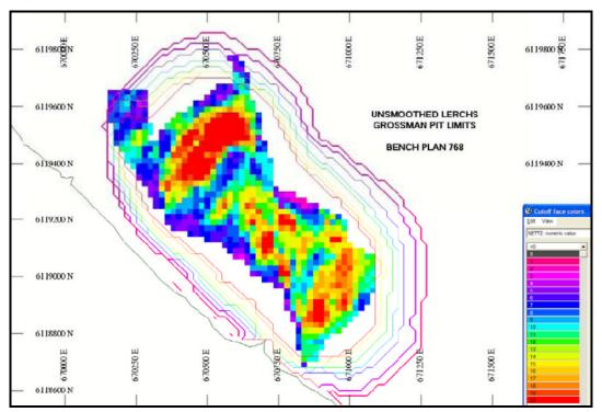
Figure 18.3 Plan View of Bench 768 Showing Pit Limits
