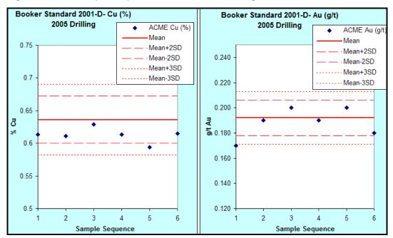
Figure 13.5 Sample Sequence Charts – 2005 Drilling Standard 2001-D
